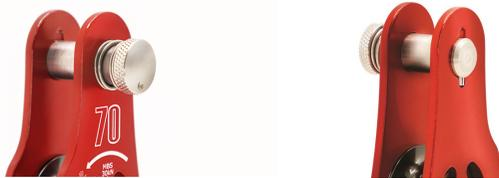
In addition to an audible click which acknowledges the location of the locking pin, the front of the pin head is marked with an indent, which allows the user to track the orientation of the locking pin, (without having to turn the device, to look at the pin-head).
