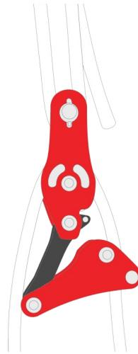
Disengaged whilst lifting load
