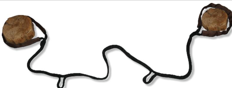
**6.** Cut the necessary length of rope. **a.** At the place of the cut, tape the rope thickly enough. **b.** Make the cut in the middle of the taping. **c.**
