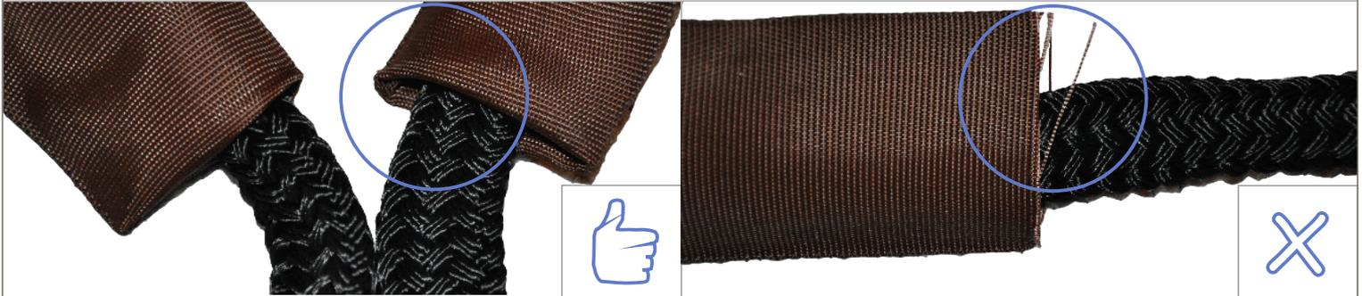
5. The first splice needs to result in the individual parts of the rope that encircle the secured trunk having an angle of  $45^\circ$  at the place of the first splice. **a.** Pull the needle through the middle of the rope so that it passes around the individual strands, not through them. **b.** Pass through both sides of the hollow rope during the first splice, pulling the inserted end through it until you reach the desired/pre-measured length.
