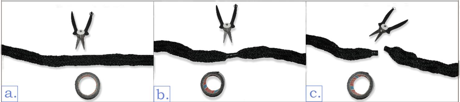
If the taping is not thick enough, the tape may not hold well, which will result in its loosening and unravelling of the end of the rope.
