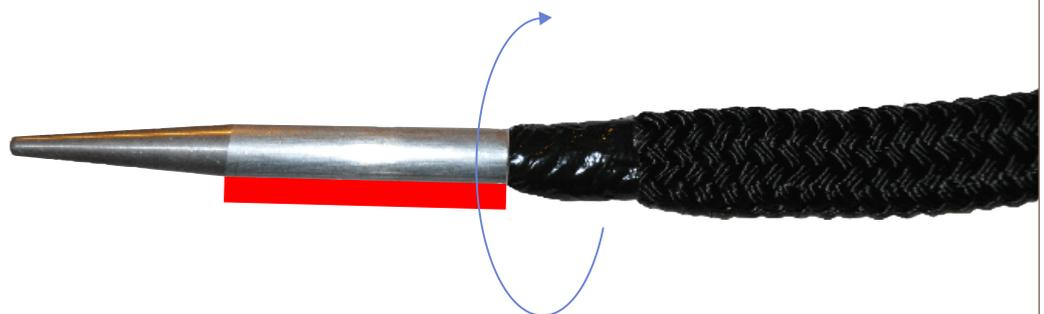
If using a long needle, attach the rope by inserting **a.** and pushing it into the opening. **b.** Then, tape the needle to the rope by winding the tape around them both a couple of times. **c.**
