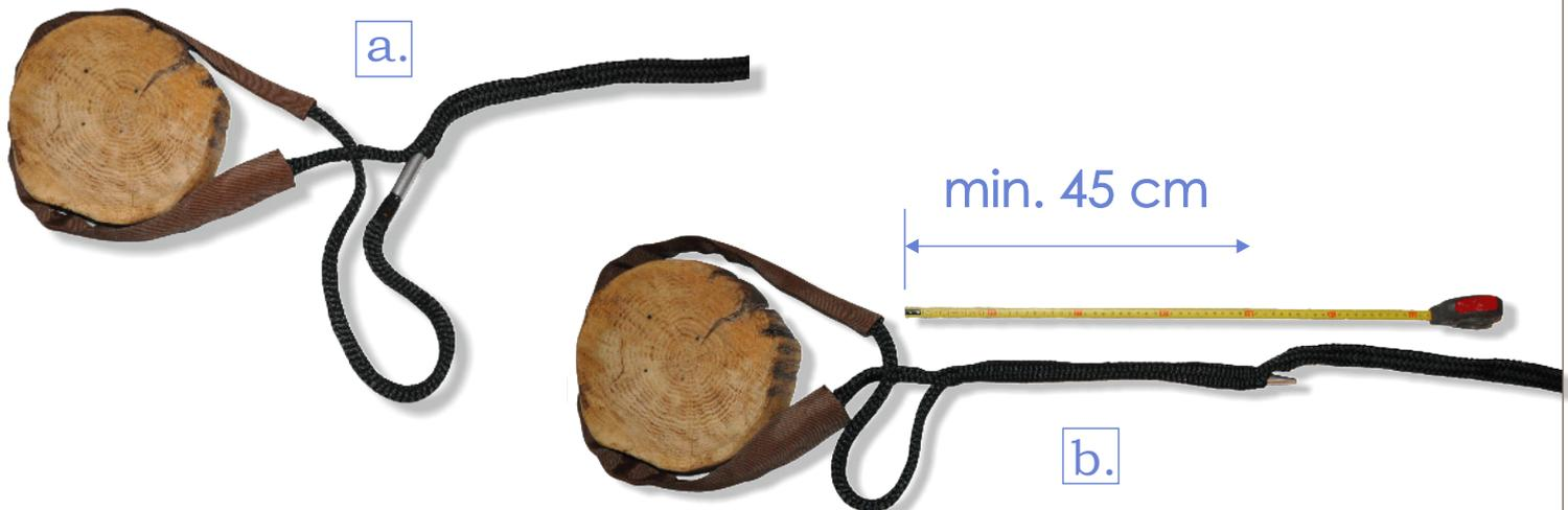
Insert the needle again about 8 to 10 centimetres **a.** below the exit point. Now, create a compensation loop. After about 20 centimetres, pull out the needle so that there will be an extra length of the loop remaining on the inserted part of the rope. **b.**
