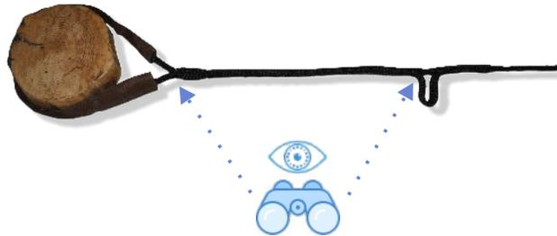
Another way of loosening the set-up in the coming years and checking its quality is to let a certain part of the rope's end hang freely behind the splicing point. This way is also adequate and provides the same functionality as the previous one; however, it might not be aesthetically desirable to leave a part of the rope at the end hanging with a knot.
