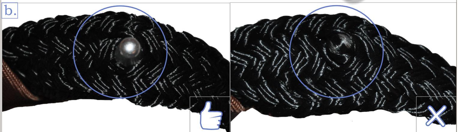
Insert the needle for the second time, about 8 to 10 centimetres **a.** below the first splice. Again, pull the needle past the individual thicker strands, not through them. Pull the needle through the middle of the rope, pulling it out after at least 45 centimetres. **b.**
