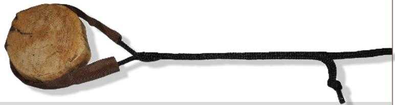
If it is not necessary to account for checks by third parties, there is no need to create a visible compensation loop at all. It is only needed to sew in enough length of the rope over the necessary 45 centimetres and keep it sewn in the rope.
