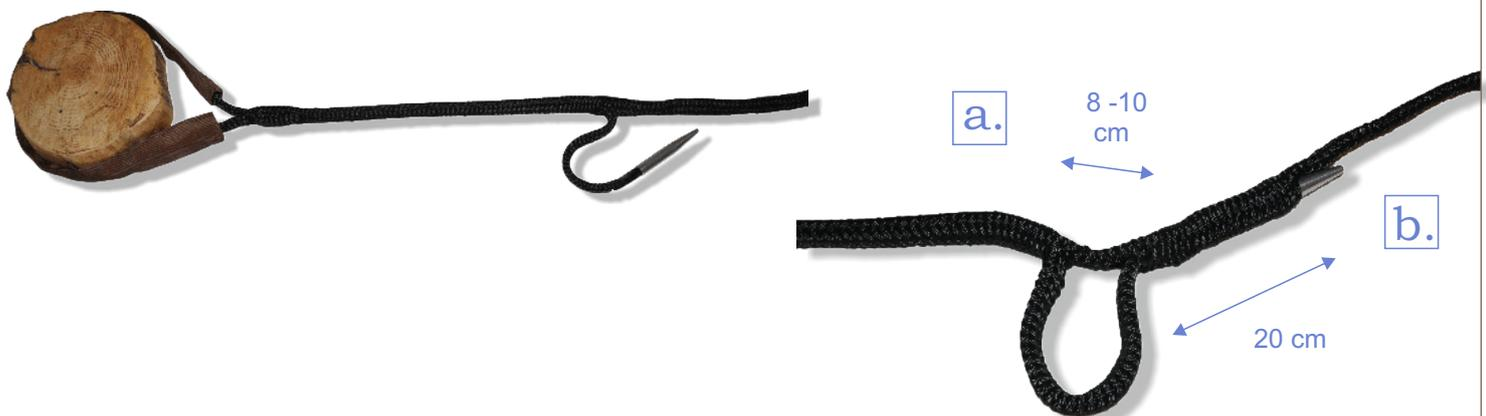
After removing the needle and taping the end of the rope that is sewn in, it will be easy for you to "hide" the end of the inserted rope into the outer rope. This way, the end of the rope will be protected against loss of the tape or unravelling of the rope itself.
